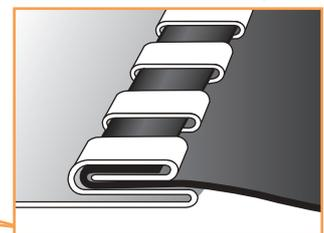
For acoustically treated ductwork and supply ducts, it is important that the fabric of the connector is also insulated in addition to the insulation fixed on the ducting. This enables the Flexible Duct Connector to achieve maximum effectiveness.
